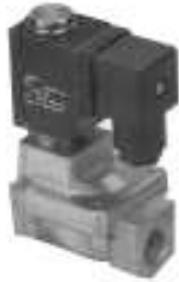
TB03EB-XXX-X Port Size: 3/8" NPT Orifice: 13 mm, 33/64" Cv: 4.5, SCFM: 126 Pressure Range: 10-150 PSI
