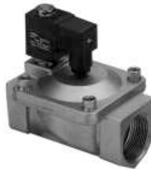
TB12JB-XXX-X Port Size: 1 1/4" NPT Orifice: 38 mm, 1 1/2" Cv: 22, SCFM: 615 Pressure Range: 10-150 PSI
